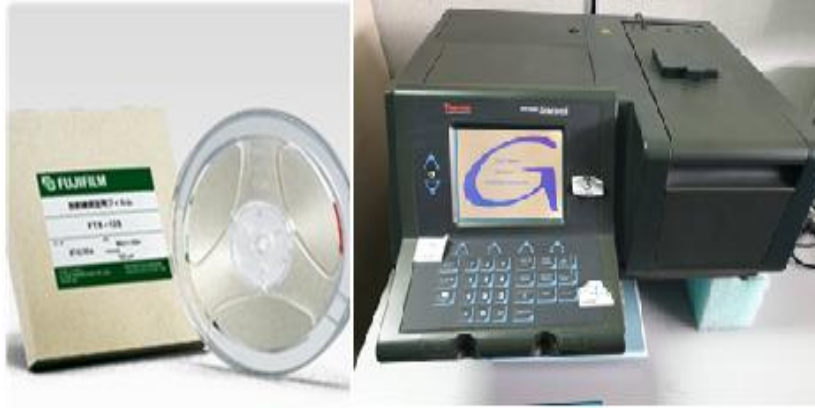
Figure 5. CTA dosimeter system: CTA film (left), GENENSYS 5 UV- spectrophotometer (right)
